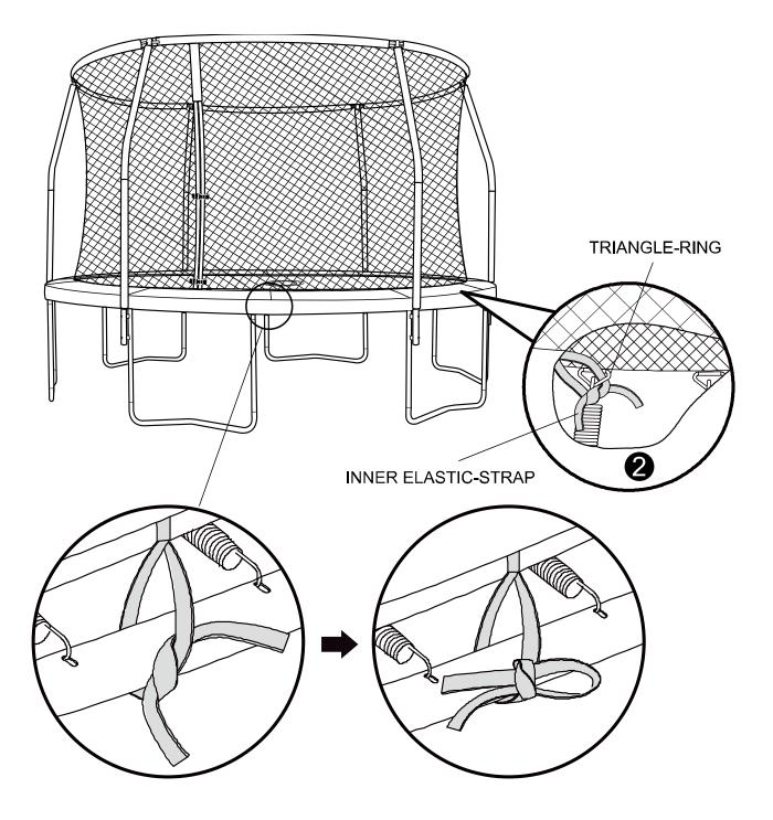
For the elastic straps near the leg sockets, wrap them BEHIND the leg sockets and then tie a one-sided bow in front as shown below.
