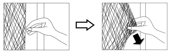
If it produces any tear or cracking or ripping sound, then the net is unsafe and MUST be taken down immediately. **STOP USING THE TRAMPOLINE ENCLOSURE IF YOU FIND ANY SIGNS OF WEAR OR TEARING ON THE NETTING.**
